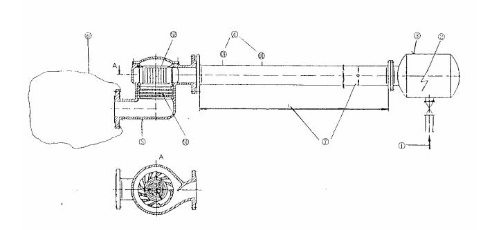
1—explosive mixture inlet; 2—ignition source; ignition within nonstreaming mixture; 3— tank; 4— measuring system for flame speed of a stable detonation; 5— flame arrester located;  $5_1$ — flame arrester element;  $5_2$ —shock wave absorber; 6—plastic bag; 7—1/d=100
