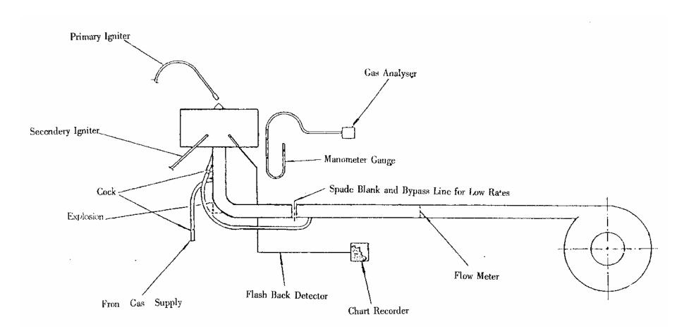
Test rig for flame arresters located in -line
